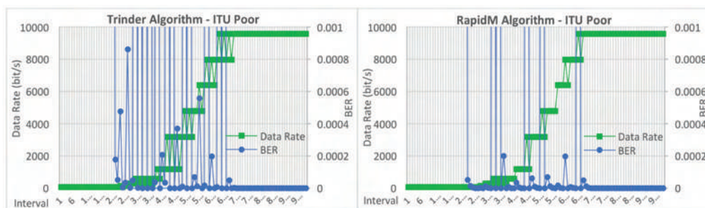
Figure 8 - BER vs Data Rate variation, for an upward SNR variation using an ITU Poor channel
