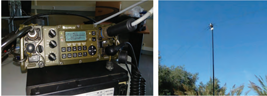
Figure 12 – E/R GRC-525 radio and RF-1936P dipole antenna
