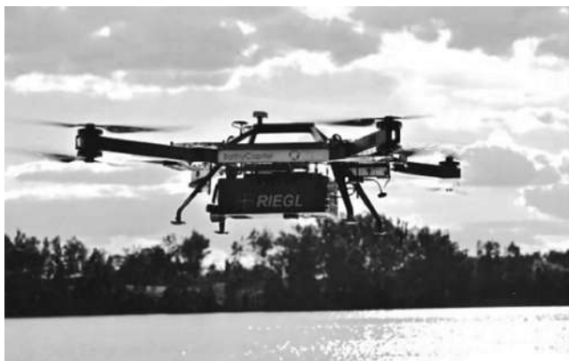
Figure 2 – UAV for topo-hydrographic data collection (RIEGL's BathyCopter)
