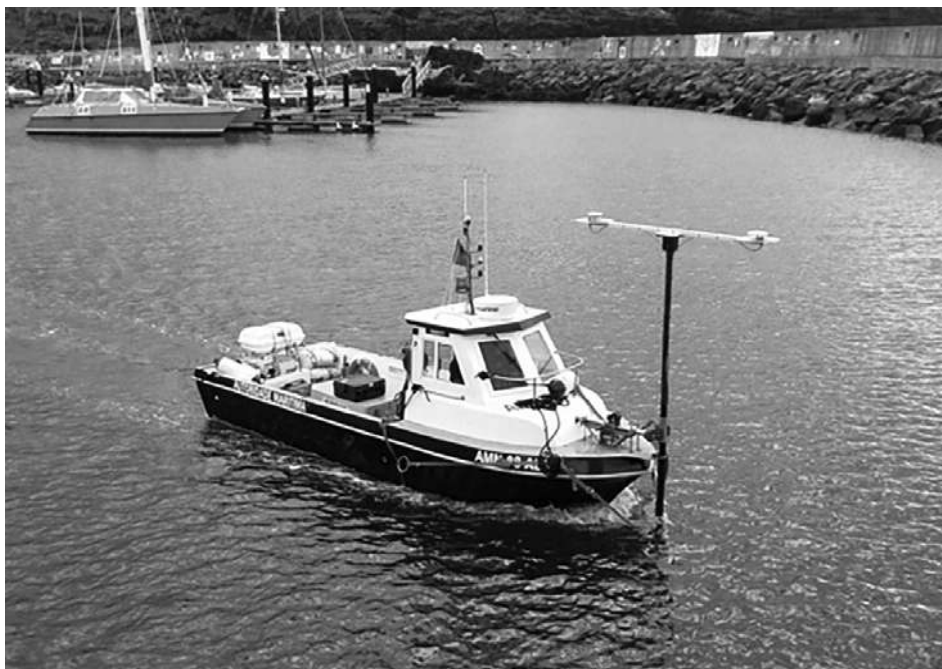
Figure 9 – Adapted survey vessel with an MBE mounted in the bow
