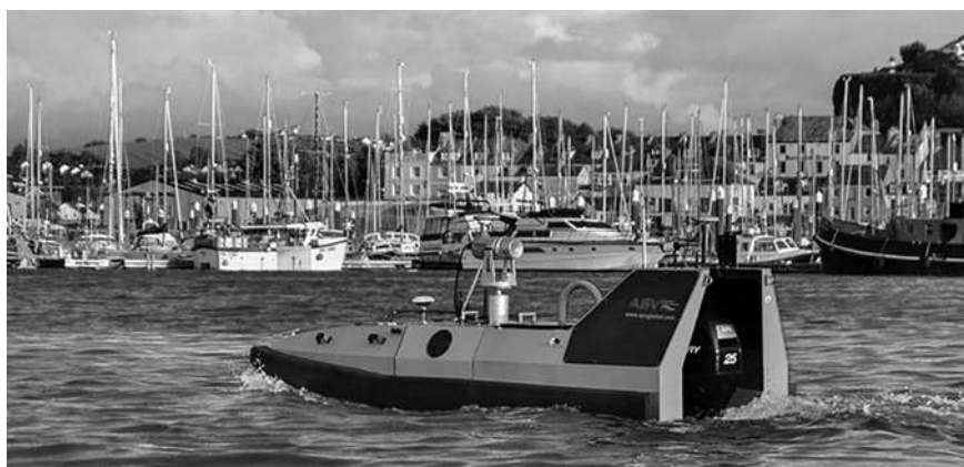
Figure 3 – USV for topo-hydrographic data collection (C-Target 3 ASV)
