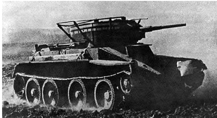
Figure 25 – A BT-5 fast tank in an exercise. The frame around the turret is a radio aerial. Both the T-26 infantry tanks and the BT-5 fast tanks had a 45mm gun that was effective as an antitank weapon and could fire a useful HE shell.
