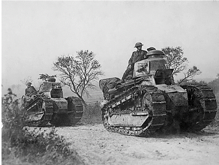
Figure 10 – Going from initial concept to mass production in just one year, and being produced in massive numbers in just one more year, the Renault FT-17 tank is a symbol of the extraordinary technological response to the problems of the Great War. Renault got the essentials of tank design right on their first try.
