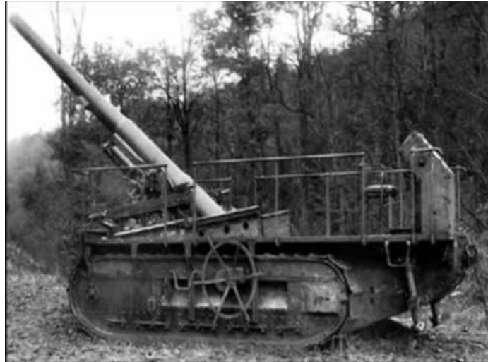
Figure 16 – A 194mm Self Propelled Gun. The successive battles concept implemented in 1918 required heavy mobile firepower, and the French Army introduced this advanced vehicle designed in Schneider's Le Creusot works that could carry either a 194mm Gun or a 280mm Howitzer. Fifty survived to see action in the Second World War.
