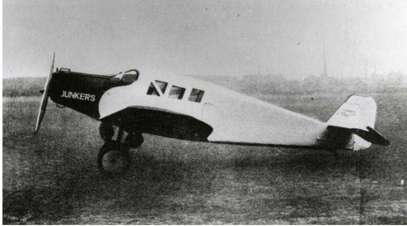
Figure 35 – The Junkers F-13, introduced in 1919, was the world’s first all metal passenger aircraft. An excellent design, it was one of the aircraft that made air travel a popular option.
