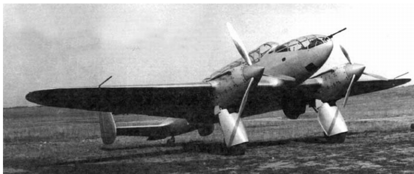
Figure 26 - A Polikarpov VIT-2 of 1937. A dedicated heavy anti-tank attack aircraft, well protected and armed with two 37mm antitank guns, the VIT-2 was the 30s conceptual ancestor of the A-10 Thunderbolt II and an illustration of the links between Deep Battle and Air Land Battle.
