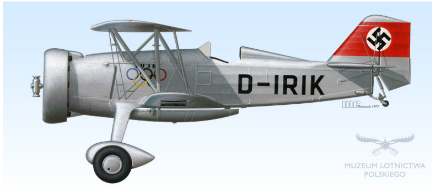
Figure 23 – An illustration of Ernest Udet's personnel Curtiss Hawk fighter bomber. The U.S. Navy and the Royal Navy had developed dive bombing as the only way to accurately hit moving ships. Curtiss had developed the Hawk II as a fighter bomber capable of dive bombing with a 250Kg bomb. Udet, then responsible for Luftwaffe procurement policy, became an enthusiast for dive bombing while flying a Curtiss Hawk, and ordered a near copy, which became the Hs123A, as an interim model, and a more developed aircraft for future equipment of the Luftwaffe. Junker's entry in the competition for the more advanced aircraft decade the famous Ju87 Stuka. Such is the myth of Blitzkrieg that many people still think the Germans invented dive bombing especially for it
