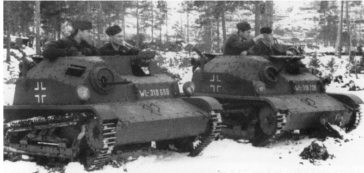
Figure 22 – Polish TKS Tankettes in German use. Conceived in the context of a possible fight against an un-mechanized force without anti-tank weapons, this vehicles proved totally useless in combat between opposing mechanized forces, wasting precious resources.
