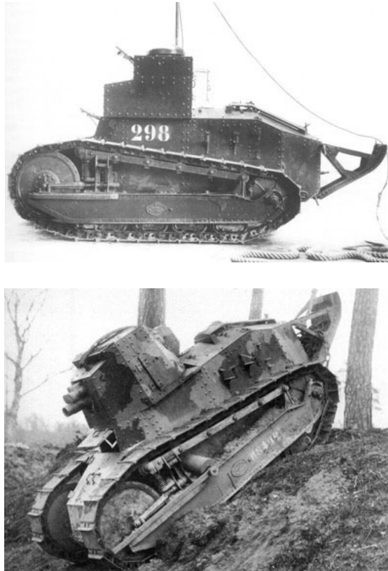
Figure 18 – The Renault FT introduced the idea of a “family” of vehicles based on the same AFV, being produced in tank (2100 built with a MG and 1246 with a 37mm gun); Assault Howitzer (39 built with short 75mm guns, shown on the right) and Radio tank (188 built shown on the left). Small numbers of other versions were built later. France produced 3177 FT tanks until the end of the war, and at the end of the war there were 2700 in the front line, total combat losses having been 439 tanks, most of which were destroyed by field guns
