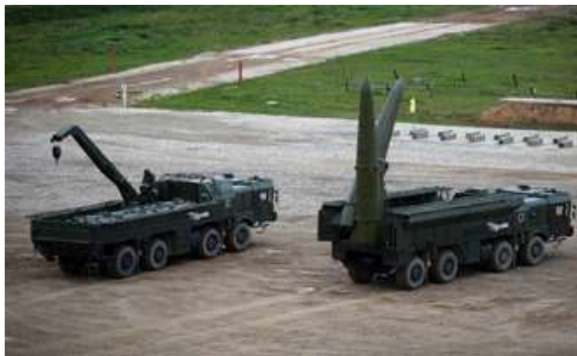
Figura 5 - O Short-Range Ballistic Missile SS-26/STONE (Iskander) : TEL e grua Fonte: Russia Military Power
