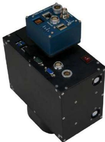
Figura 2 – Sensor multiespectral micro CASI 1920
